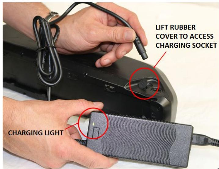
**⚠ CAUTION** - Only use the charger provided to charge your eTrike battery. Using the incorrect charger may damage the battery and would invalidate your warranty.
