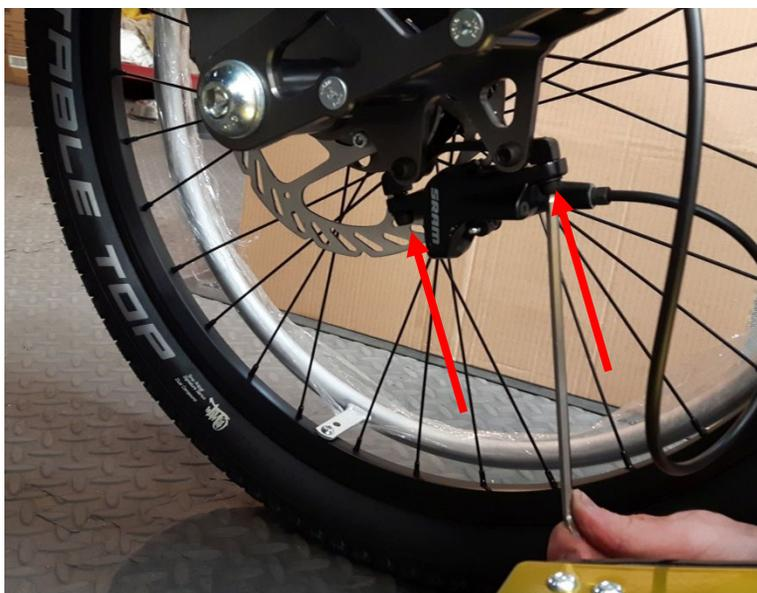
1. Using a 5mm Allen Key, loosen the 2 vertical calliper bolts. This allows the calliper to 'float' sideways
